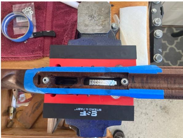
Step 4) Strip the action of everything that is below the bottom surface of the action. Then use modeling clay (I get mine from Michaels). Fill all holes in the bottom surface, then use a chisel to cut the clay off smoothly. Note the front of the action where the set screws for the barrel are I put some blue painters tape over the allen head of the set screws and then held it in place with the modeling clay.
