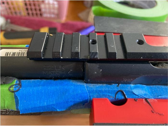
Here you can see how the epoxy swished out in the wells. This is where I could test if it was set up.
