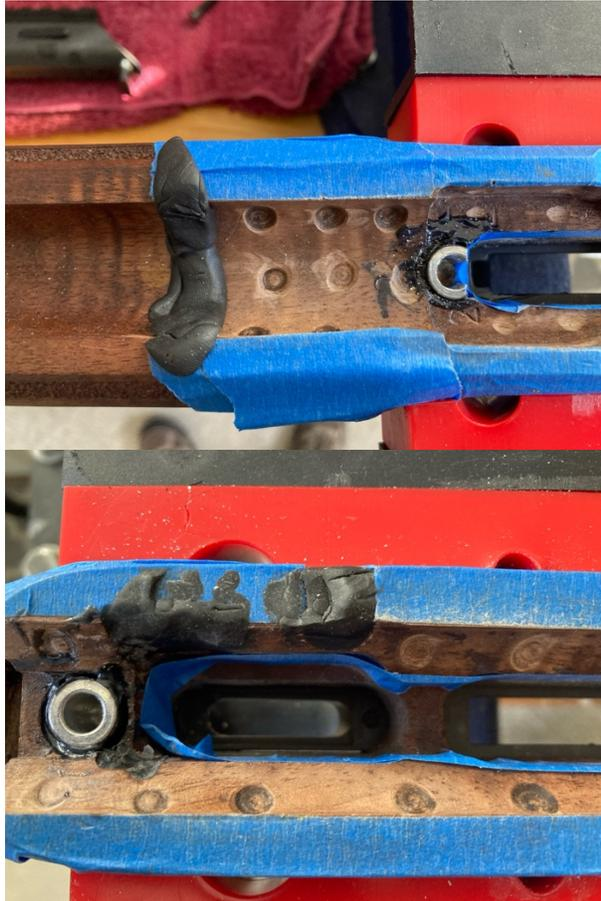
Also put something in the front of the barrel channel to help keep the barrel centered. I used paper towels but wish now that I had used layers of painters tape on the barrel that would have done a little better job.
