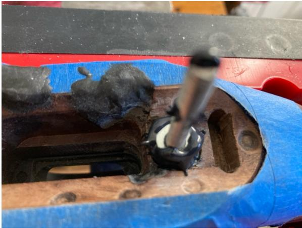
g). Now I took the spacing board and put it on, put on a washer on each screw and added a nut and then tightened slightly each screw so that the total assembly was solid against the bottom of the stock.
