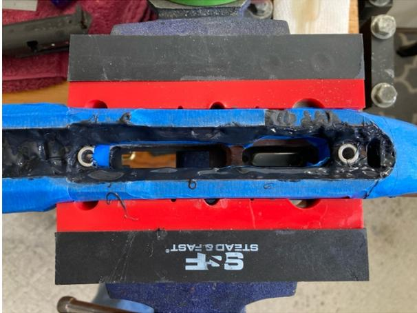
At this point I put the action screws back in and tightened them to about 10 lb-inches. If things went well you will have epoxy squishing out all around the action and the front inch of the barrel. Here is where you need a ton of q-tips to clean the break line all up. The cleaner you get this step the better things will be. I am not too worried here because it is after I get this bedded right I will refinish the stock. But...
