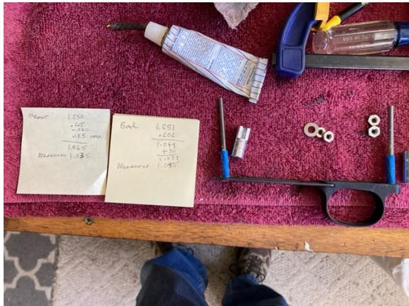
c) now take the pillars and put them over the tape, Then put a #10 washer and thread a nut all the way down and tighten. This should make the pillar stand up hard and perpendicular to the plates inside edge. Careful not to get wax on the outside of the pillars,
