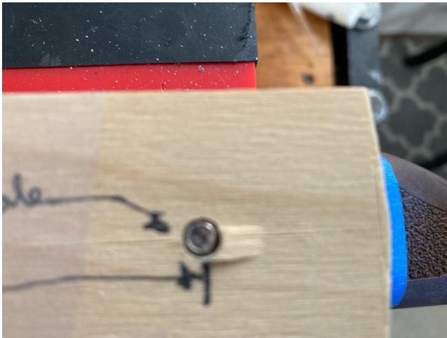
e) Assuming all is well, we now mix the epoxy. Not a lot but I used a 3oz bathroom cup to mix about 3X what I did the first time. Then I took my small screwdriver and got some epoxy and applied a thin coat to the walls.
