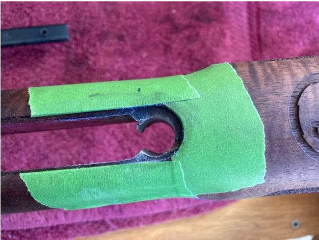
Now that the holes are drilled you need to check centering. Put the bottom metal back in and stand the pillars on top of the bottom metal. Then measure with your calipers to the surface of the inlet next to the pillar. We want that value to be .030 when we have filed the bottom surface of the pillar, not the top that mates to the action. We want that to be perfectly flat because the bottom of the action is perfectly flat.
