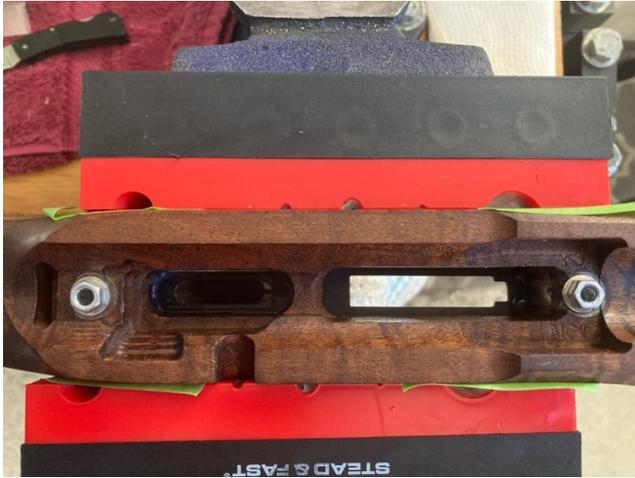
That is it for the first gluing. It will be set up but not hardened (4-6) hours. This will allow me to trim any excess off if needed.
