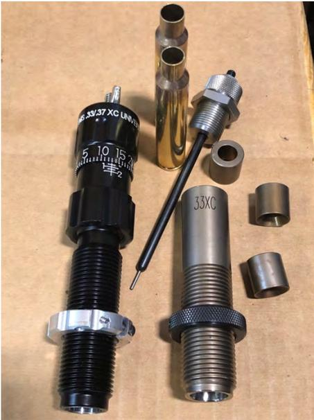
For reloading on the Dillon 550, the seater needs to be shorter by about .375" (either 33XC, 37XC, or 41XC). If you are going to load on a Dillon 550 then let Katie at Superior Shooting Systems know and we will send you a modified 33XC/37XC/41XC seater die at no charge.
