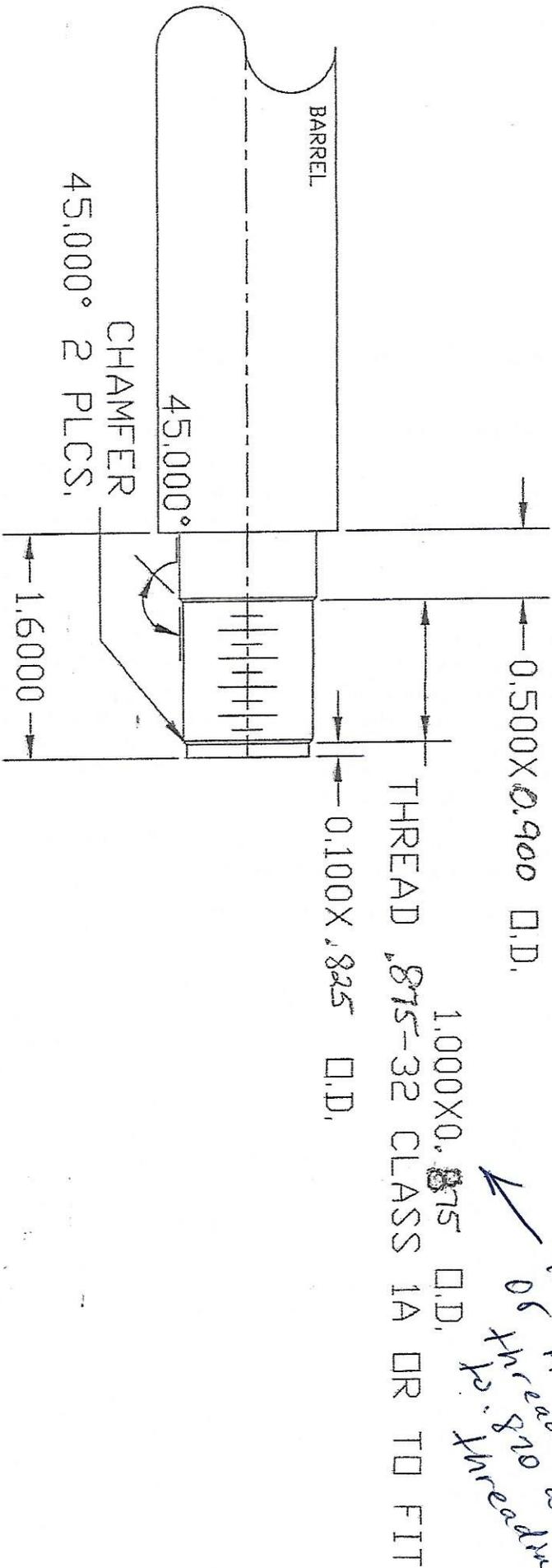
NOTE: For Unified Inch screw threads there are six standard classes of fit: 1B, 2B, and 3B for internal threads; and 1A, 2A, and 3A for external threads. All are considered clearance fits. That is, they assemble without interference. The higher the class number, the tighter the fit.
