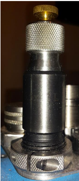
"Floated," custom, full-length, non-bushing sizing die = 0 runout
