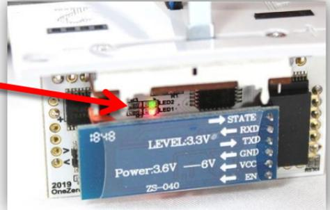
Once you are sure there are no lights, unplug the scale power cord and install the jumper wire as shown.
