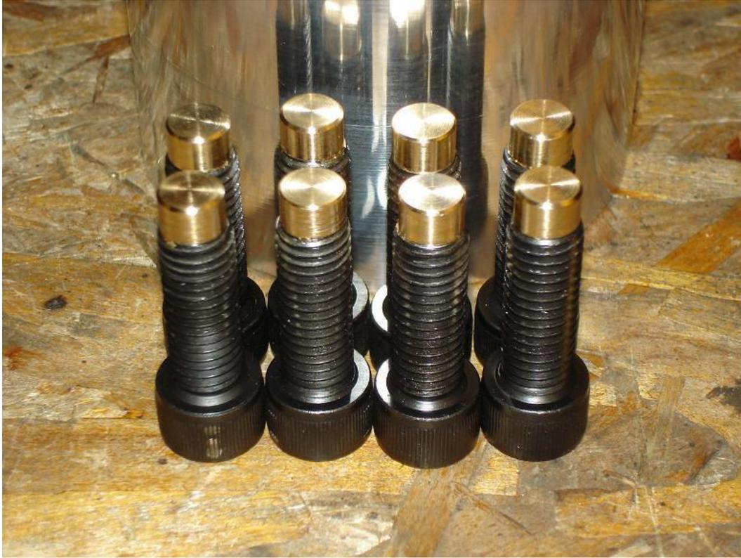
and while I am posting pictures, here is the fixture I made to true my action. it is basically the same idea as the barrel through the headstock.
