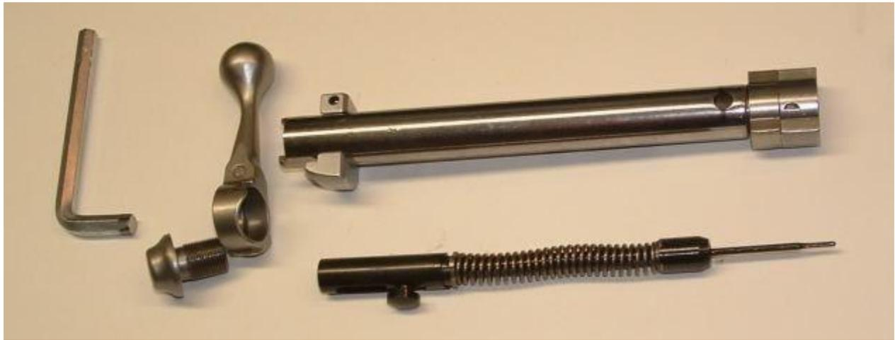
**STEP 2: REMOVE BOLT HEAD PIN**
