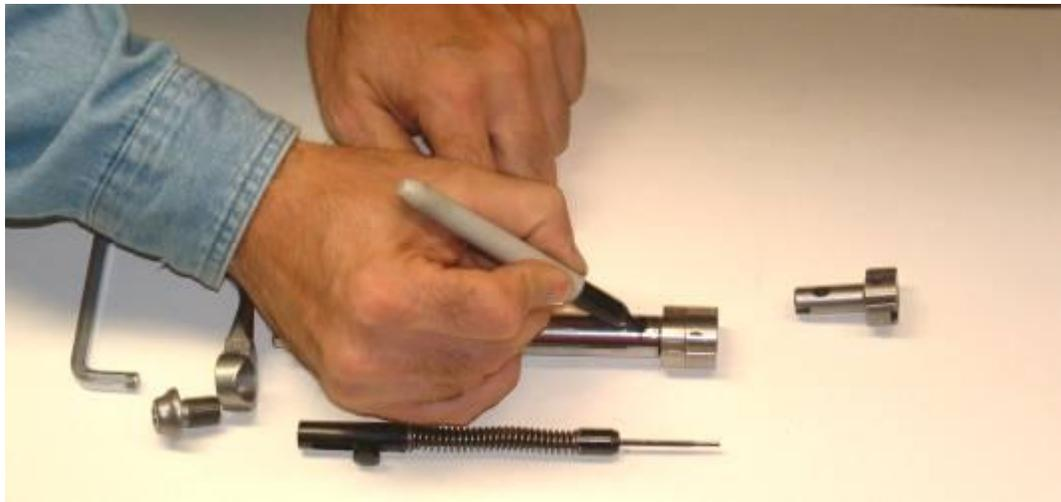
Mark the position of the pin in the bolt by drawing a line with a permanent marker on the bolt through the pin.
