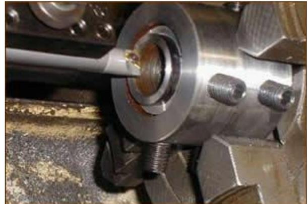
Set-up to face the receiver locking lugs.
