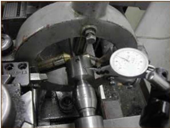
Adjusting steady rest to true bolt face. The dial indicator is to check that the bolt body doesn't move when steady rest points are adjusted.
