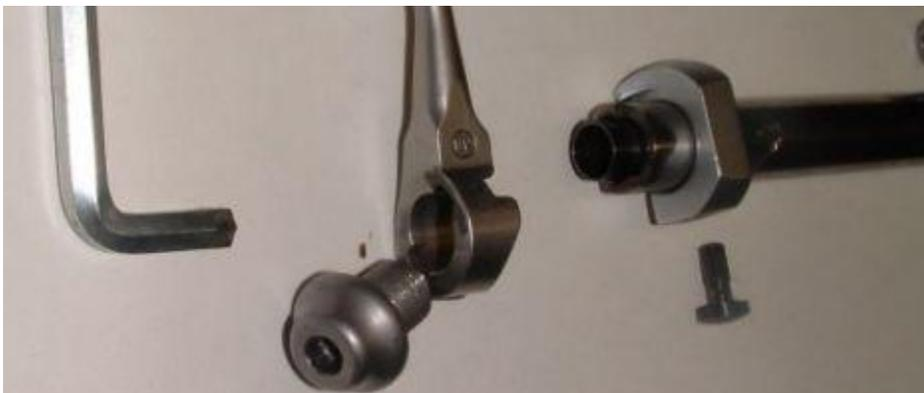
With the pin removed, the striker assembly can now just slide out.
