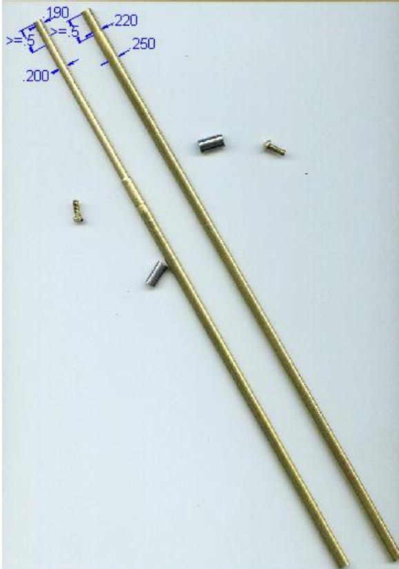
You'll notice that there is a step in the smaller rod I will probably turn it down to .200 the rest of the way down the rod until there is only about 1" left unturned so the rod isn't trying to flex in to places.
