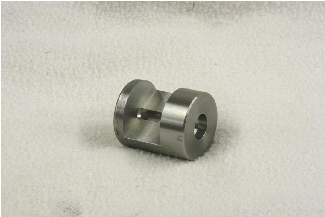
A gage made from a short section of barrel stub left over from crowning. The chamber reamer is run in about 0.250, with the throat area revealed using an end mill. Used to measure the amount of shoulder bump-back when body or full length sizing, as well as to check the seating depth to the lands for different bullets.
