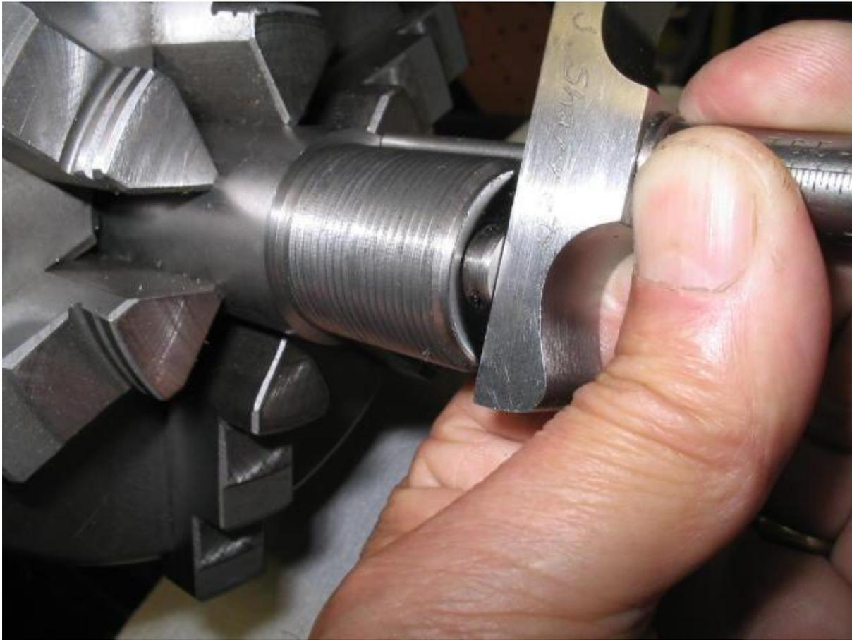
It is almost impossible to get an accurate headspace reading since the micrometer will cock over and give a false reading.
