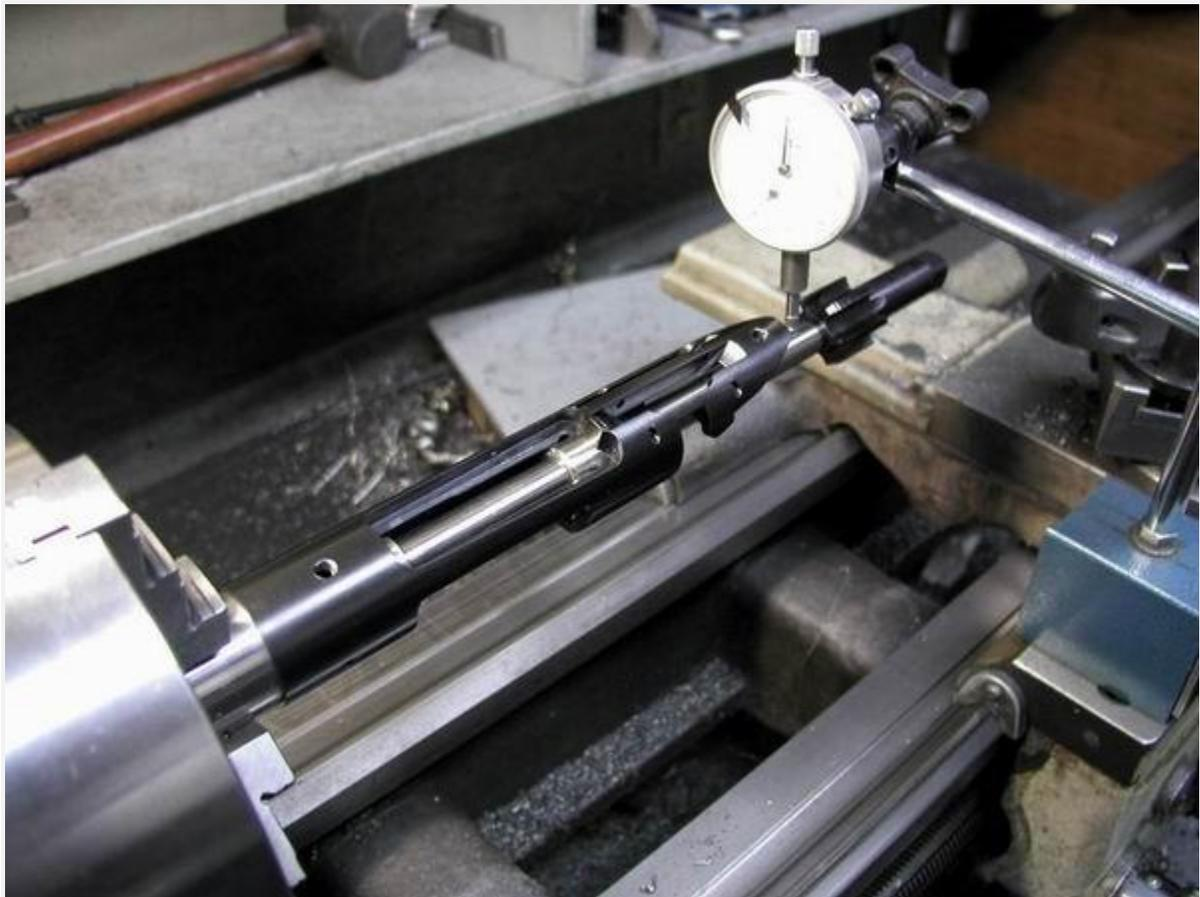
This is a picture showing although the front and one lug recess are faced true it still needs more facing as the other lug recess is untouched...
