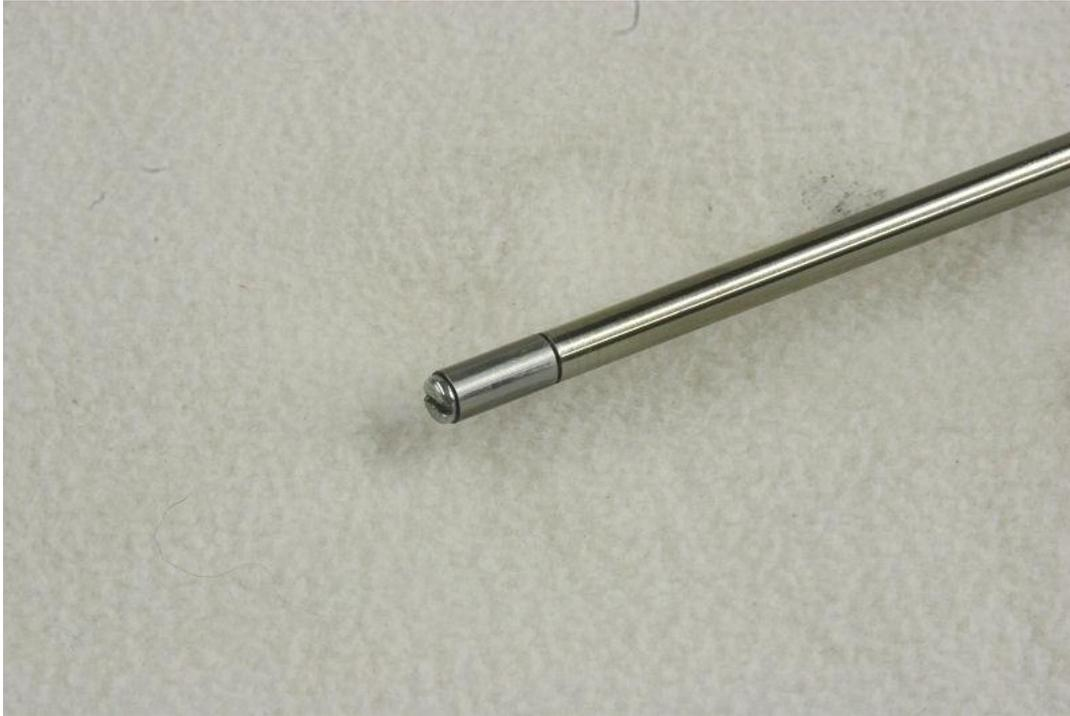
Another view of the 6mm rod, showing the 6mm bushing installed. The 4-40 screw holds the bushing in place.
