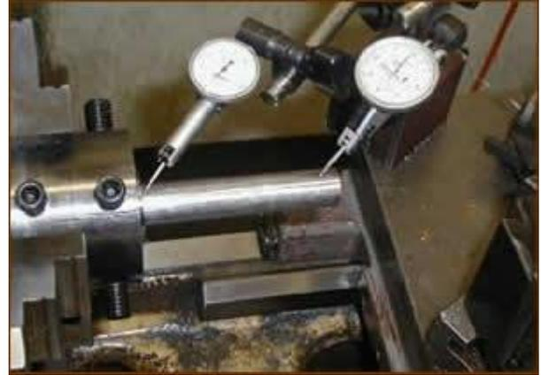
Indicating the receiver bore for minimum run-out. A tight fitting mandrel is a necessity.
