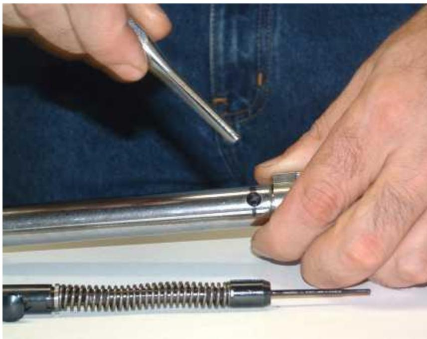
By pushing the bolt head in towards the bolt it should be possible to push the pin out of the bolt.
