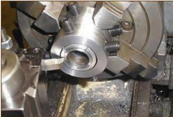
Facing the front of the receiver. The receiver is held in the indicating collar.
