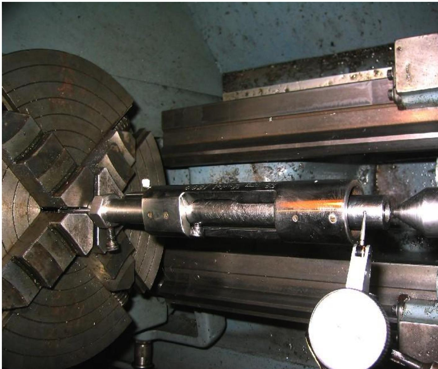
In this shot we are attempting to improve on a factory action - in this case the Japanese Howa. A custom mandrel must first be ground-up to closely fit the bore of the action. The action is prevented from rotating on the mandrel with the small socket-head screw in the port. Another ring-clamp prevents it moving towards the chuck. The mandrel is 'clocked'
