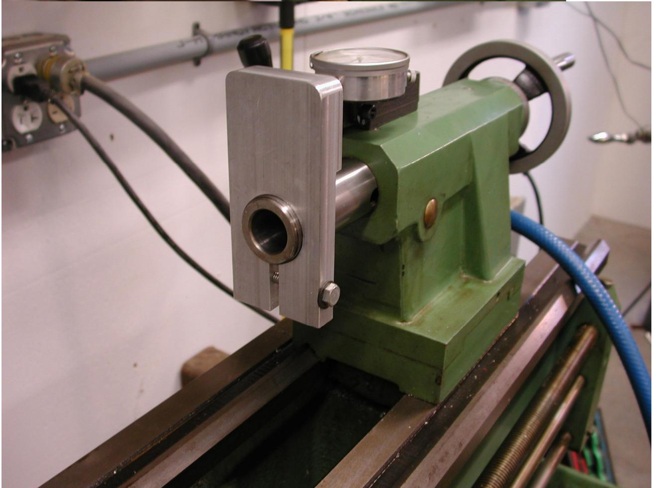
This is the "Cat Head" or Spider I made to go on the back end of the spindle.
