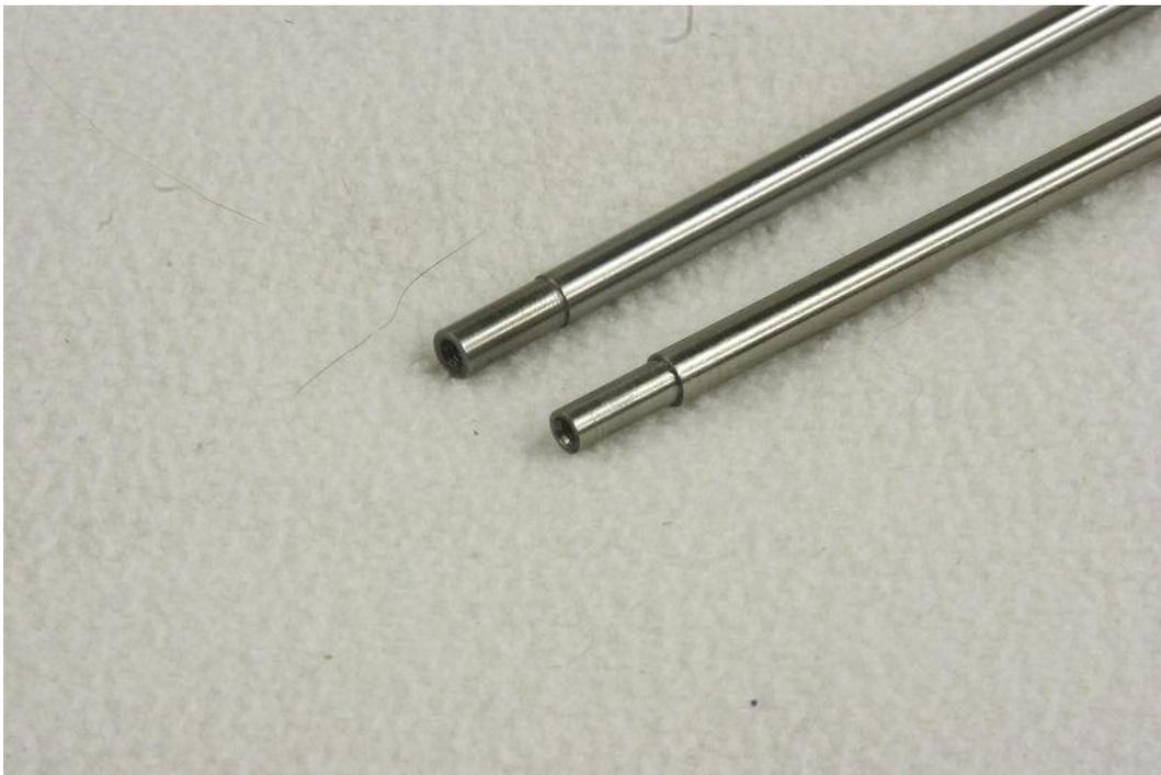
Another view of the rods, showing the 6mm and 6.5mm bushing surfaces. These are machined to a perfect slip fit, with less than 0.0001 clearance. The 6mm rod is made of 303 stainless turned down to 0.232, and the 6.5mm rod is made with 0.250 W1 drill rod.
