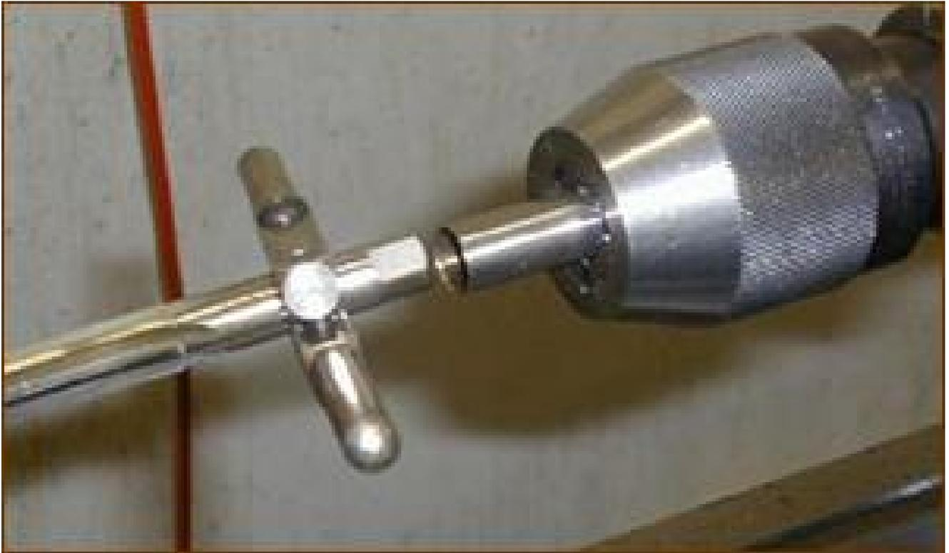
The Simple Reamer Holder. The holder is bored .020" oversize of the reamer shank.
