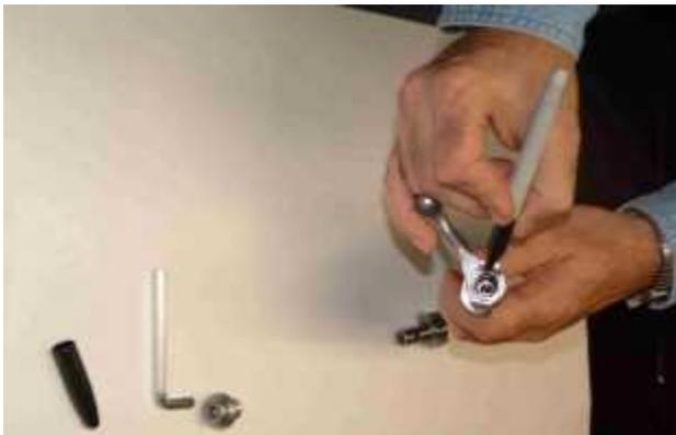
The bolt shown above has an Allen (Hex) type bolt assembly screw. Older models are provided with a simple slot. Unscrew it all the way out. You may want to mark the bolt handle and body to simplify reassembly.
