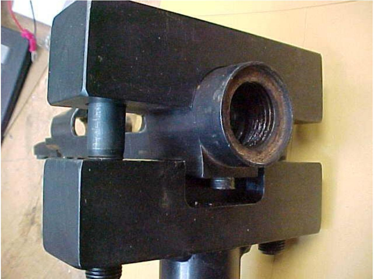
This shows the Brownells action wrench in action. If the action was blued, an aluminum shim could be wrapped around the top half of the action. But, take note of the cutout portion of the handle that allows for the recoil lug. If not for this cutout, the wrench could be made from a solid bar, with two holes, tapped or not, for the bolts.
