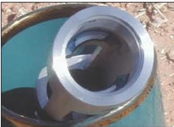
The end result of precision machining. Full contact of both locking lugs without lapping on this receiver. If lapping, is required after truing, it will take a very minimal lapping to
