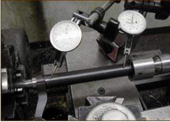
Indicating in bolt body. The bolt is held with threaded ball similar to a construction ball.
