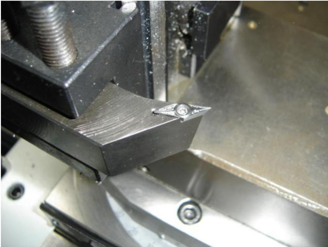
The .004 radius insert is a Kennametal polished carbide high speed aluminum finishing insert.
