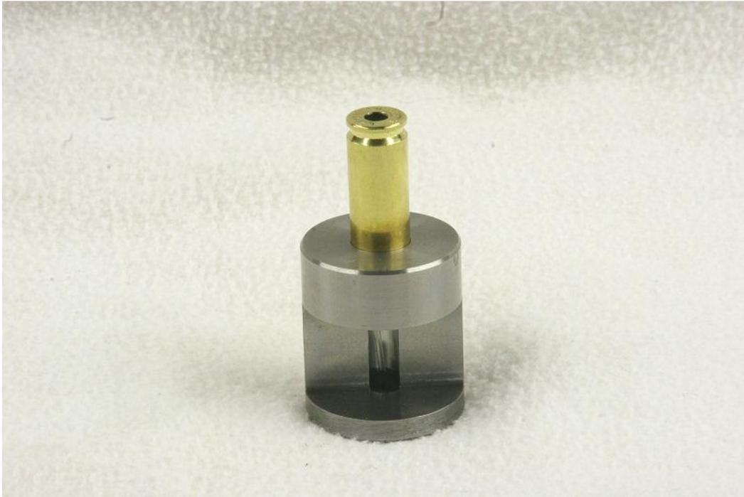
Another view of the headspace measuring gage, showing a 6 Dasher case in place.
