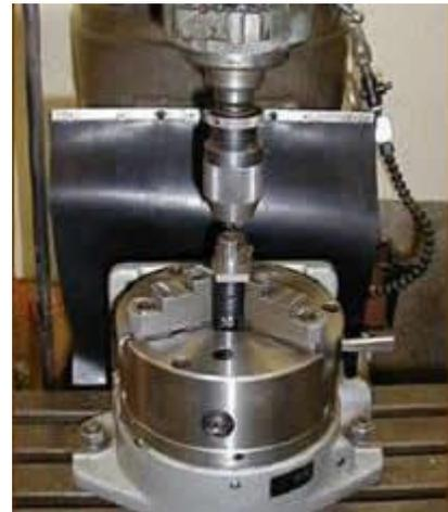
Drilling receiver to pin Holland recoil lug.
