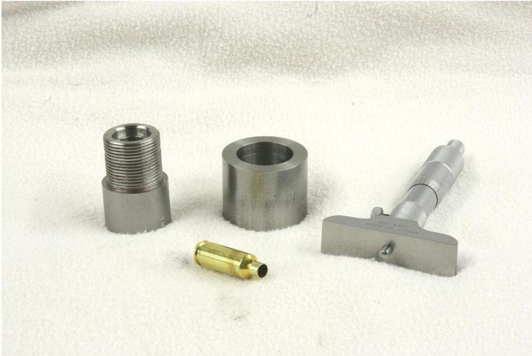
A precision gage made from mild steel, exactly 1.2500 in. long, and a slip fit over a standard Remington 1.060 thread tenon. Used to assist in measuring the protrusion of the go-gage during chambering and headspacing. Avoids having the depth micrometer rock on the back of the go gage.
