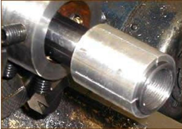
This shows the collet that is placed around the receiver to keep from marring the finish of the receiver.
