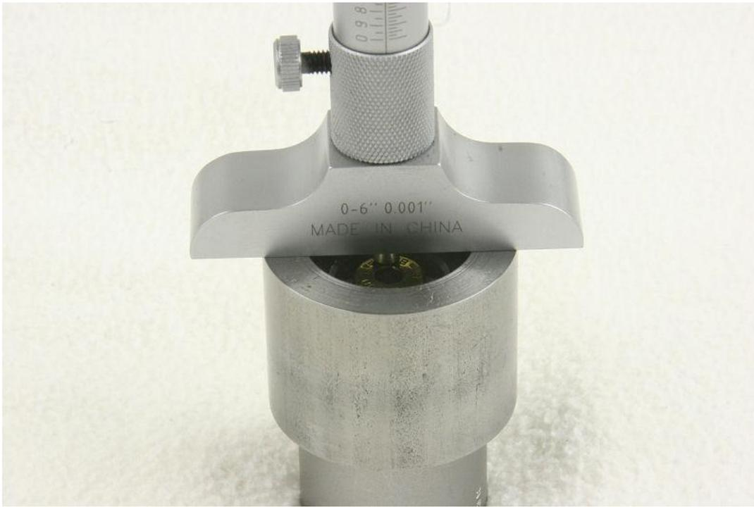
Another view of the headspace measuring collar, showing it in place over a chamber and tenon section in 6 Dasher left over from a barrel set-back. A 6 Dasher case is used to illustrate the process.
