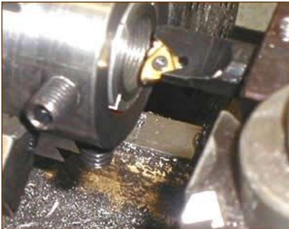
Single point re-cutting the receiver threads.
