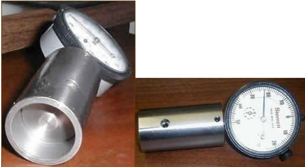
Pictured above is the tool that I use for measuring the cone on previous barrels. Also, can use it for a direct reading off a headspace gage.
