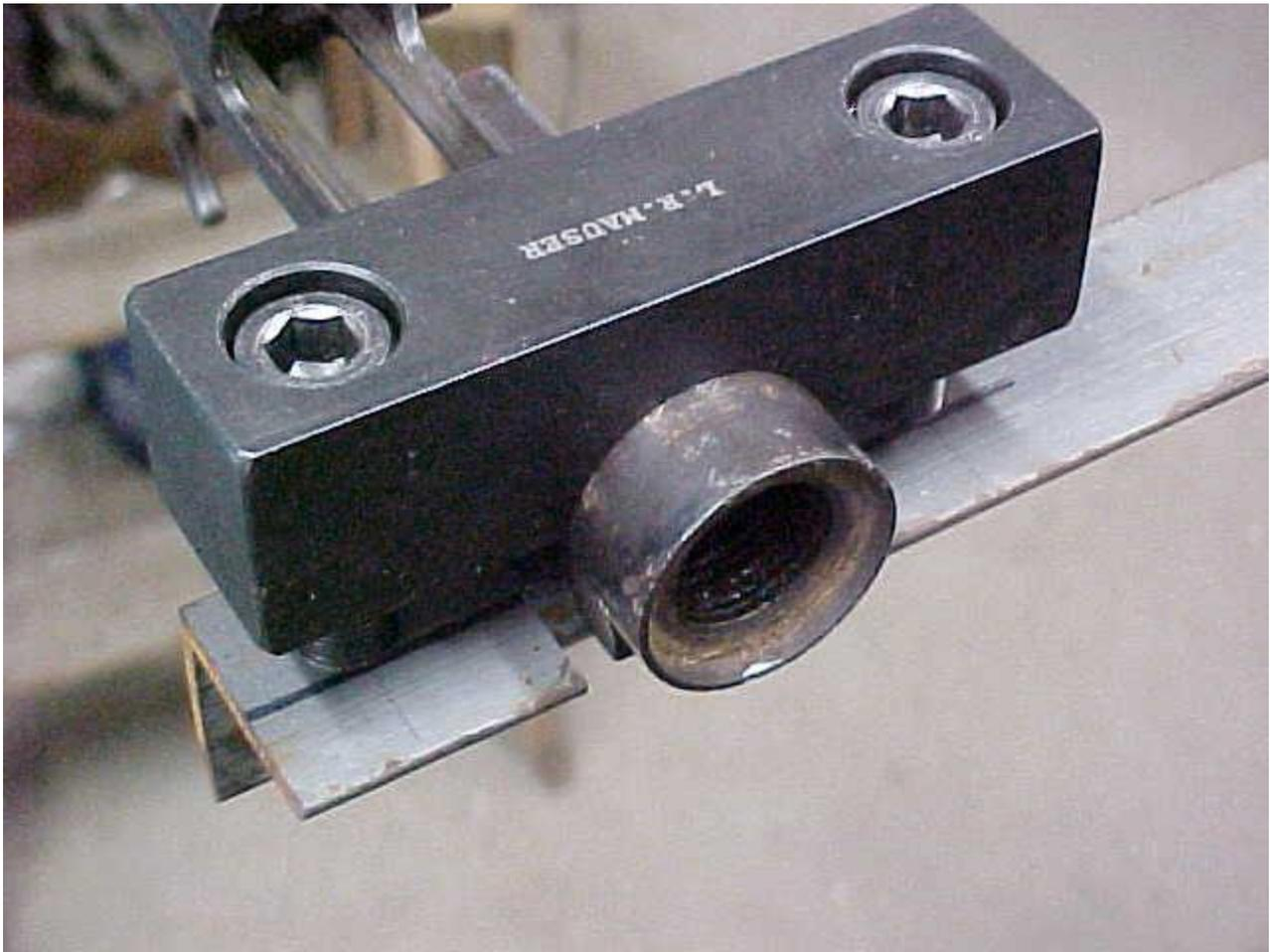
This shows the "economy" handle, just a piece of bedrail, with two holes and a notch. This one is about 3 feet long with the action at the end. If your bench/shop will stand the extra length, use a four foot piece and but the action in the middle. Then two of you can use it, one on each end.
