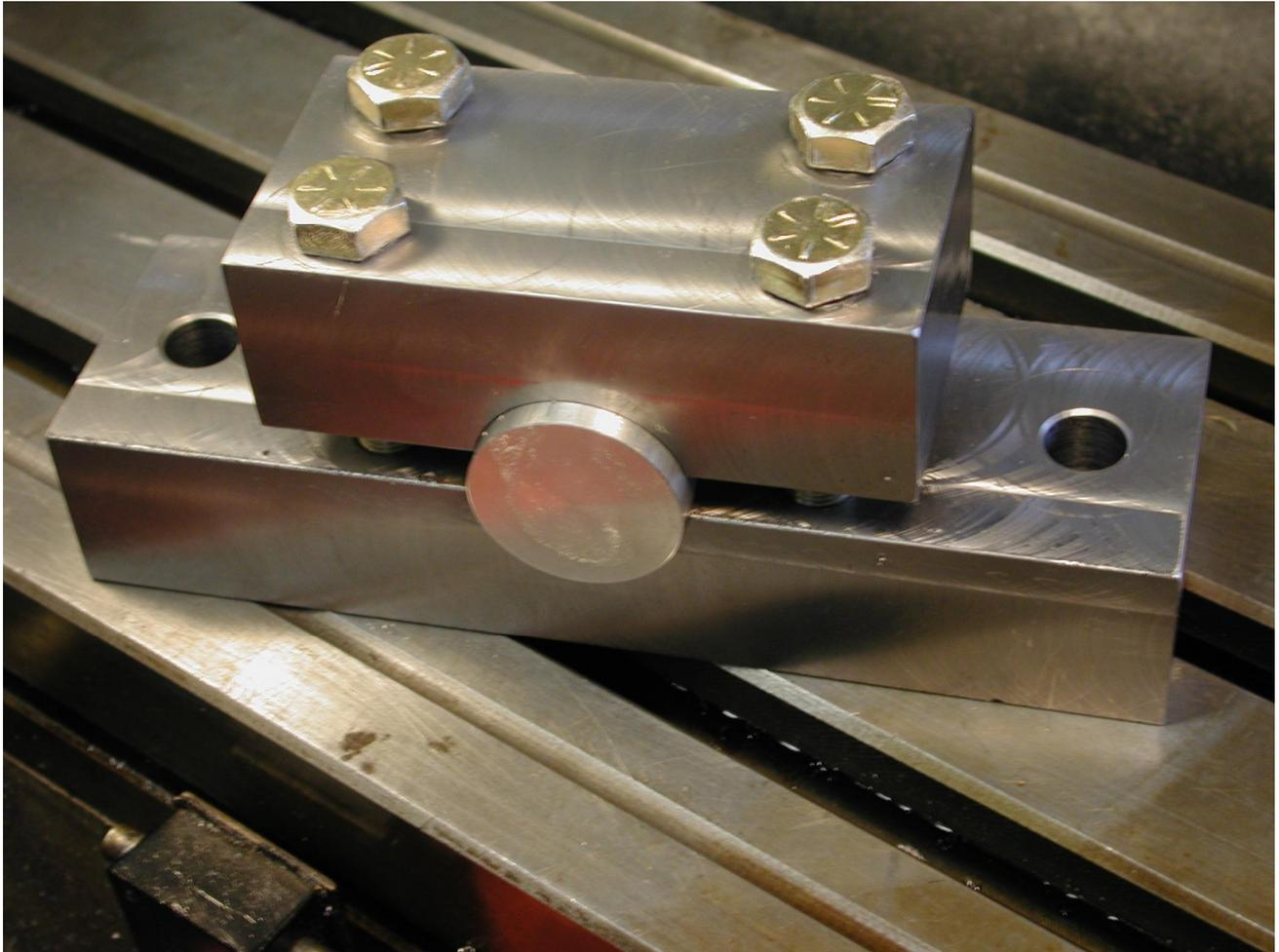
The mounting holes were drilled 9/32" to use 1/2" mounting bolts. The base piece is 8" long.
