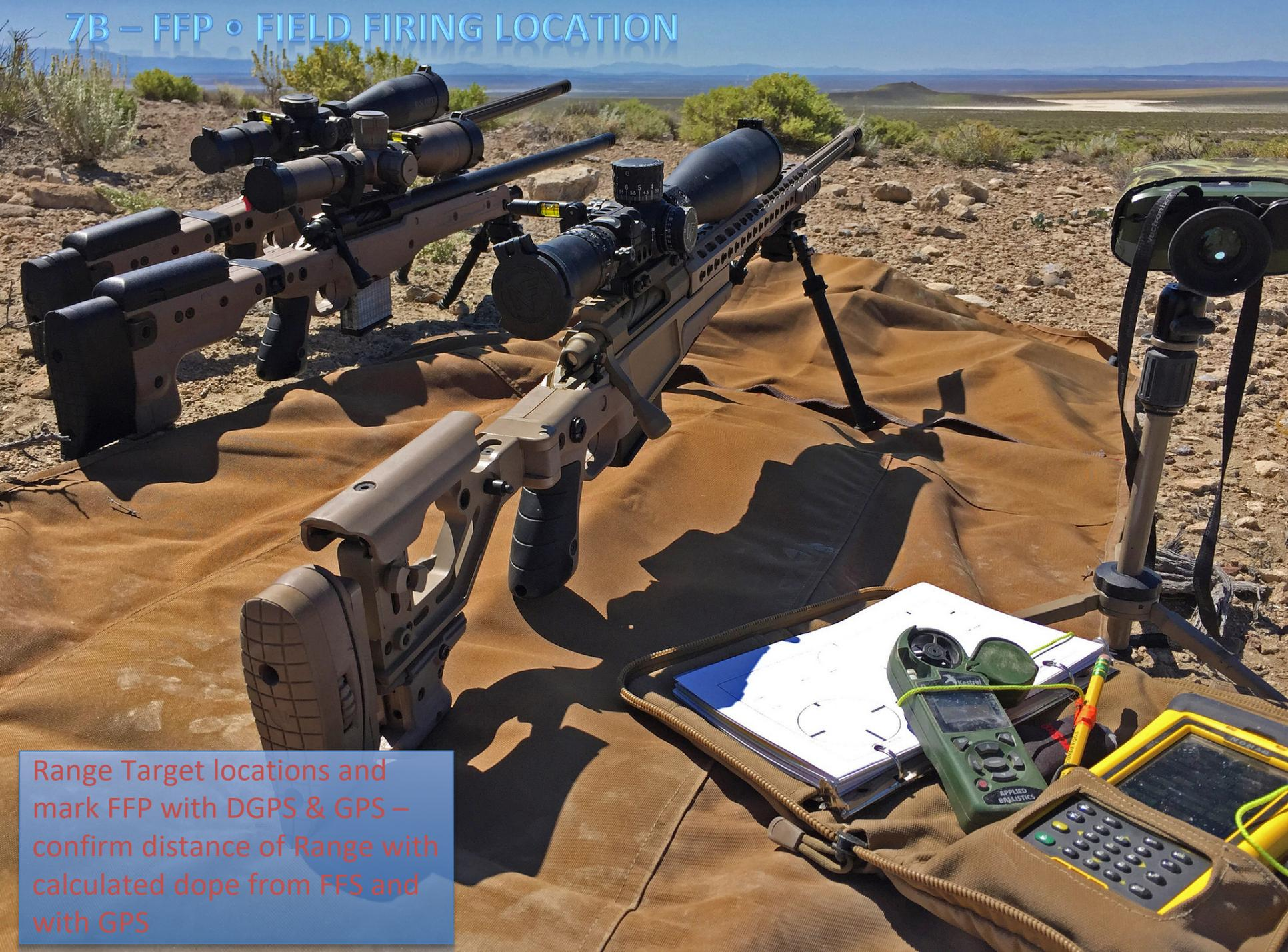
Range Target locations and mark FFP with DGPS & GPS – confirm distance of Range with calculated dope from FFS and with GPS
