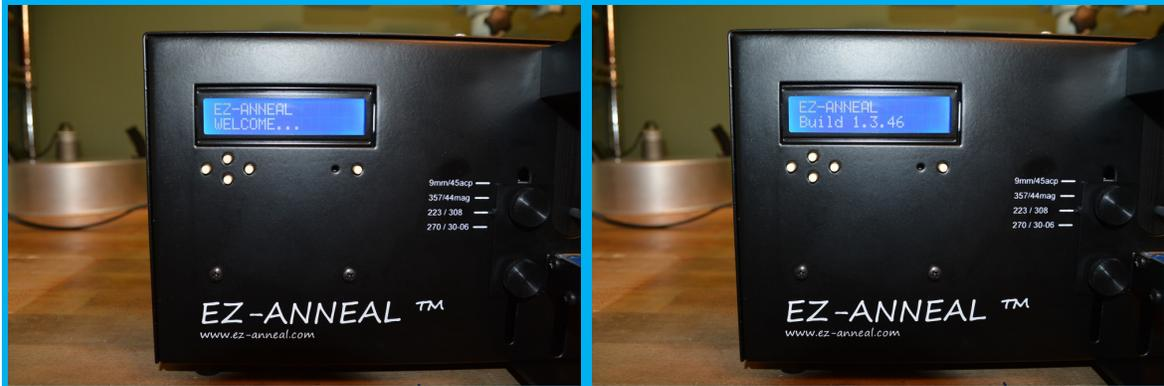
5. Next the system will prompt you to press the Select Button. The Select button is located at the right side of the LCD Display. Button presses should be quick and deliberate. **Avoid holding the select button in, or you may jump through the next menu inadvertently.** A simple tap is all that's required.
