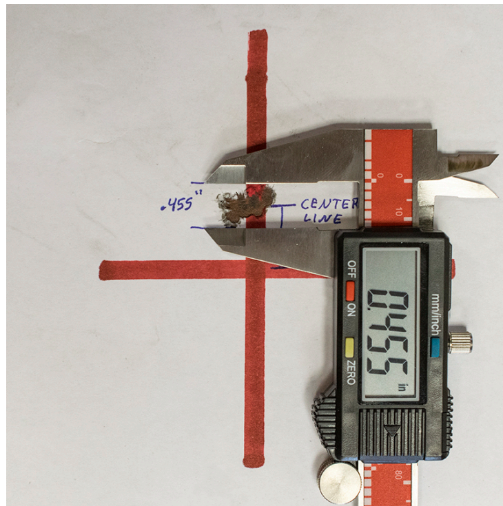
Figure 6: Vertical Impact Point Measurement, Individual Holes Not Visible
