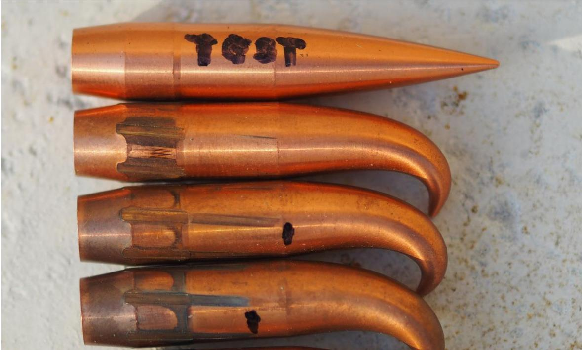
With proper base-drilling, the rearmost aperture-sealing portion of the rear driving/sealing band becomes a thick-walled cylindrical pressure vessel for which Lamé's Equations can be used to calculate internal stresses and radial displacement as functions of the base-pressure  $P$  ducted internally.
