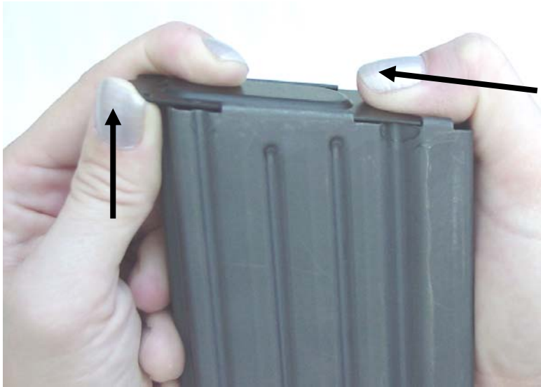
Figure 2-5b Removing Magazine Base
