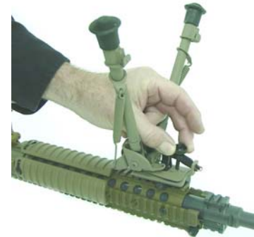
2. Tighten Bipod Nut.
