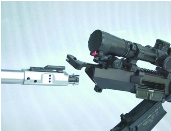
2-7 d. Withdraw Bolt Carrier Assembly
