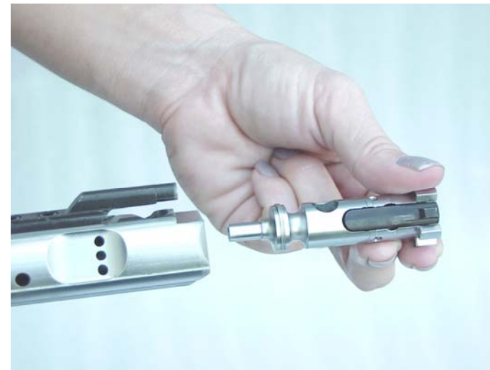
2-8 d. Remove Bolt Assembly
