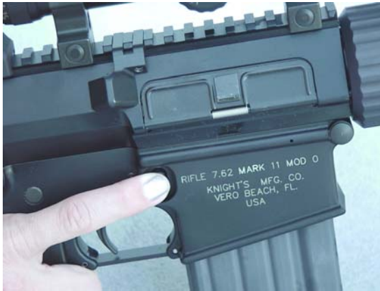
2-7 a. Release Magazine and Clear Weapon
