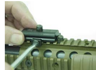
4. Ensure Adapter screw is tight.
