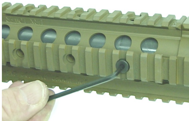
3. Remove screws from both sides. (Note: as many as 6 screws may be present.)
