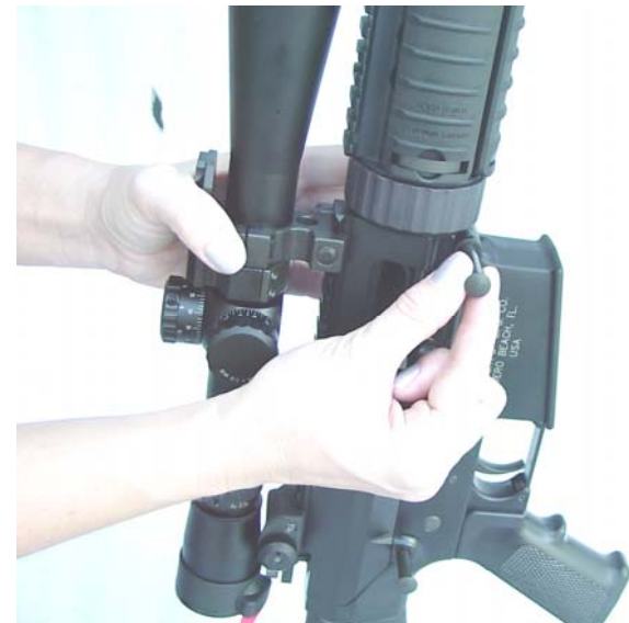
2-7 f. Pull Front Pivot Pin
