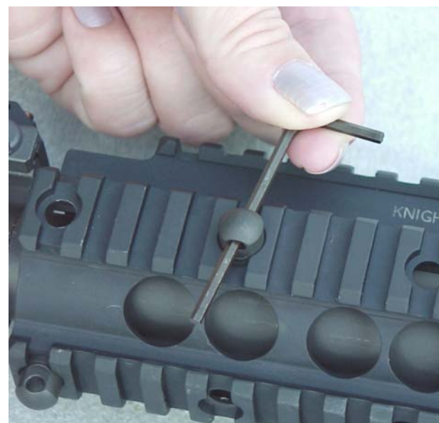
d. Tighten with allen wrench.
