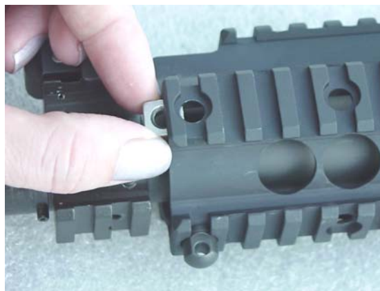
a. Slide nut into channel.
