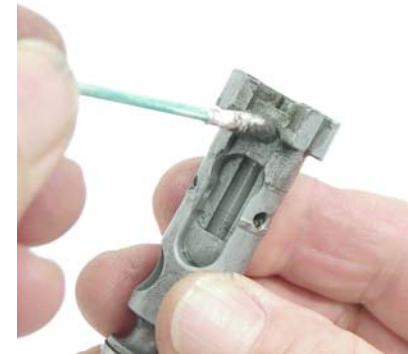
Q-Tips for Extractor & Cam Pin Recesses
