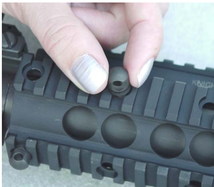
c. Screw stud into nut.
