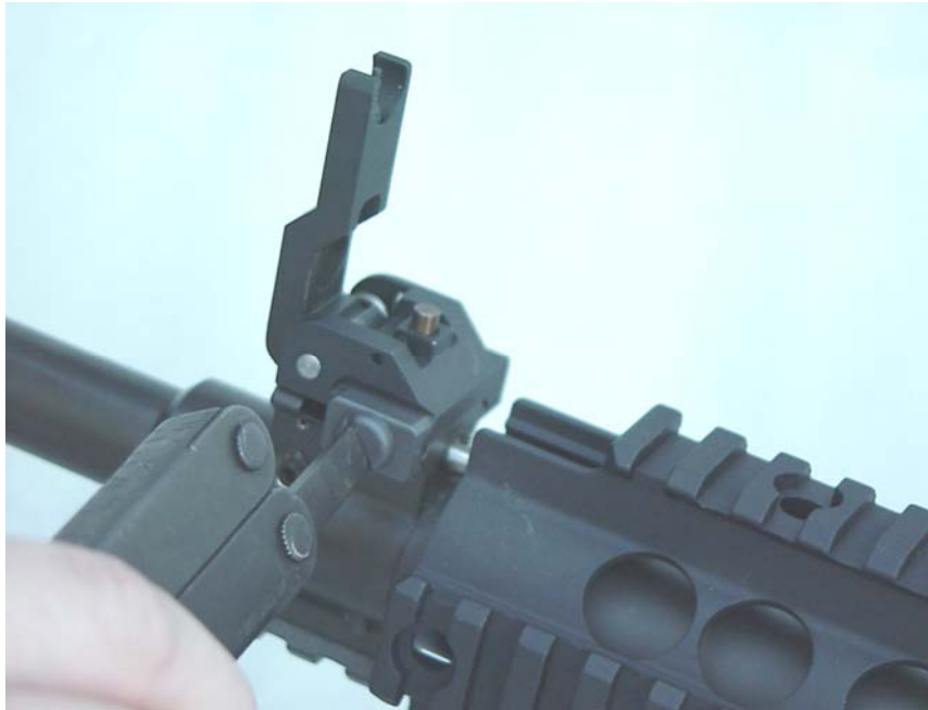
Figure 2-6 Installation of Mk 11 Back-Up Front Sight
