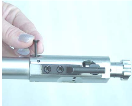
2-8 b. Pull Firing Pin Retainer Pin
