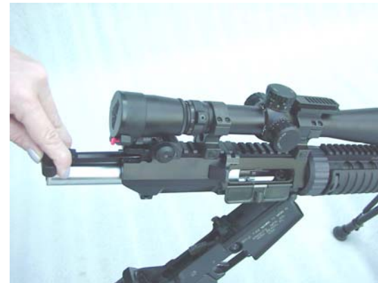
2-7 c. Slightly Retract Charging Handle
