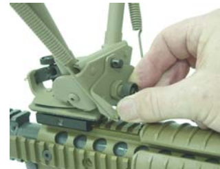
3. Tighten Bipod Pivot Tension.
