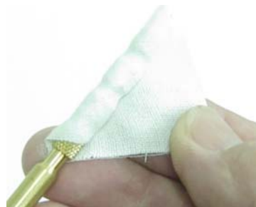
Wrap patch tightly around jag before insertion.
