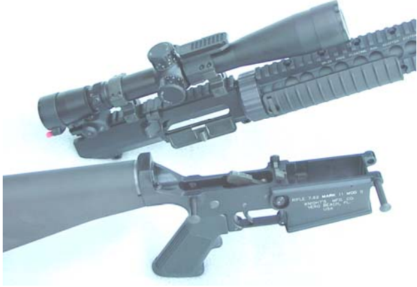
2-8 a. Separate Upper and Lower Receivers
