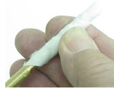
Wrap patch tightly around jag before insertion.
