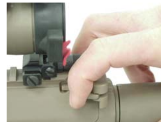
Moving scope forward may improve charging handle access.
