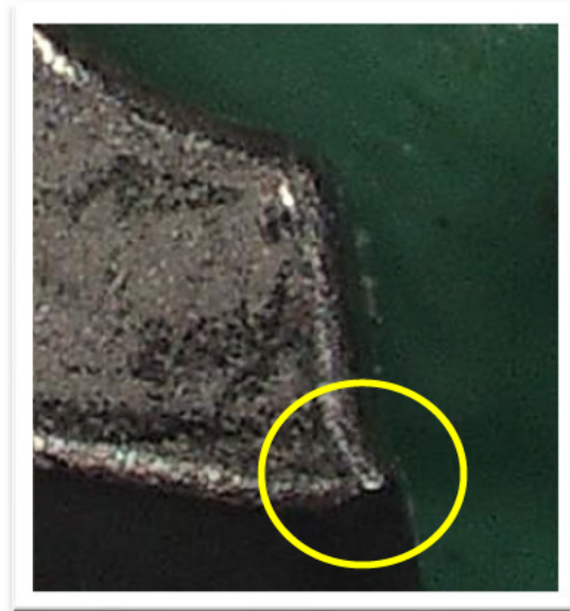
Figure 18- Subject Firearm Striker Pin Hook "Ledge"
