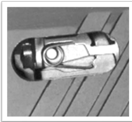
Figure 30 - Striker Safety Lock (up position)
