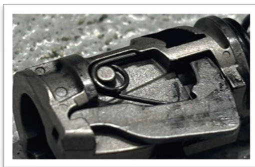
Figure 24- Post-Firing Spring Position
