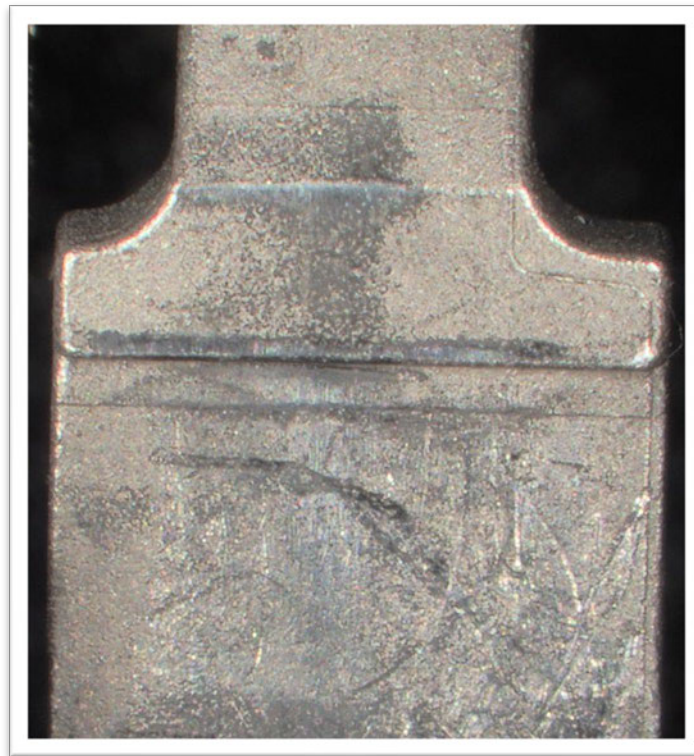
Figure 16- Wear on the Primary Sear Notch 18
