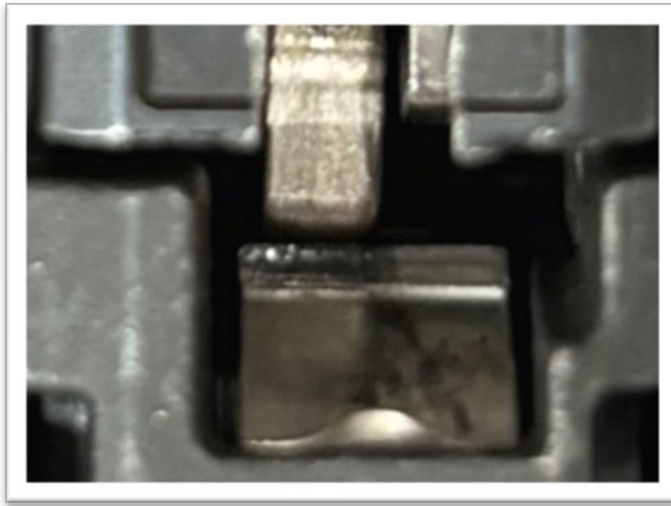
Figure 34 – Striker Hook Placement on Secondary Notch
