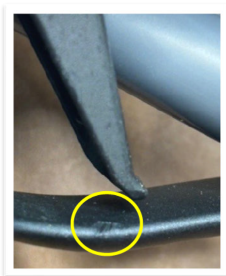
Figure 13- Trigger Guard Abrasion
