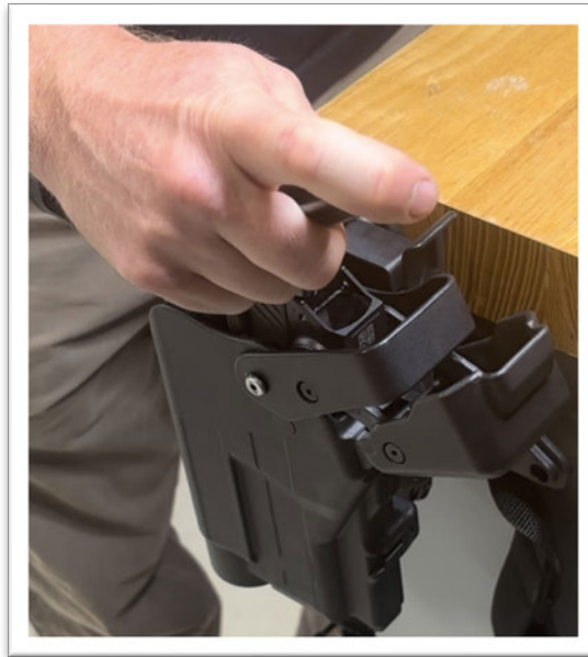
Figure 36 - Striker Safety Lock Test (no manipulation)
