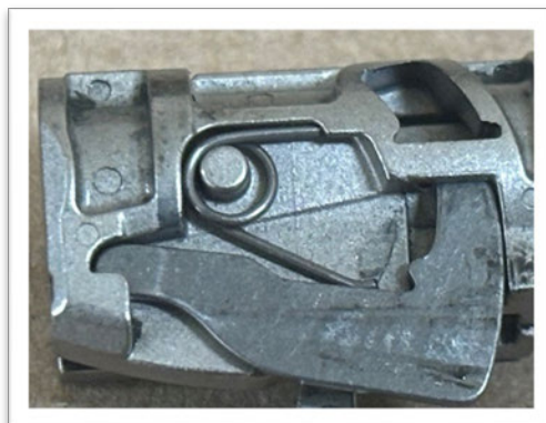
Figure 23- Pre-firing Spring Position
