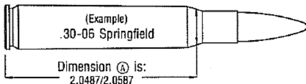
The zero on the headspace gauge represents the minimum number of dimension A.
