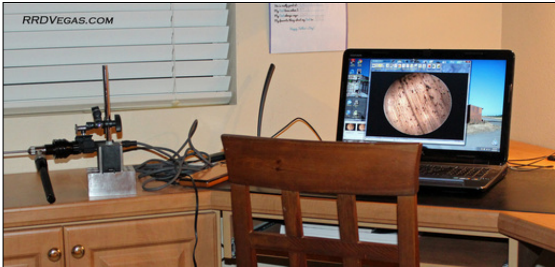
Inspecting the barrel on the computer with the attached Sony video camera.
