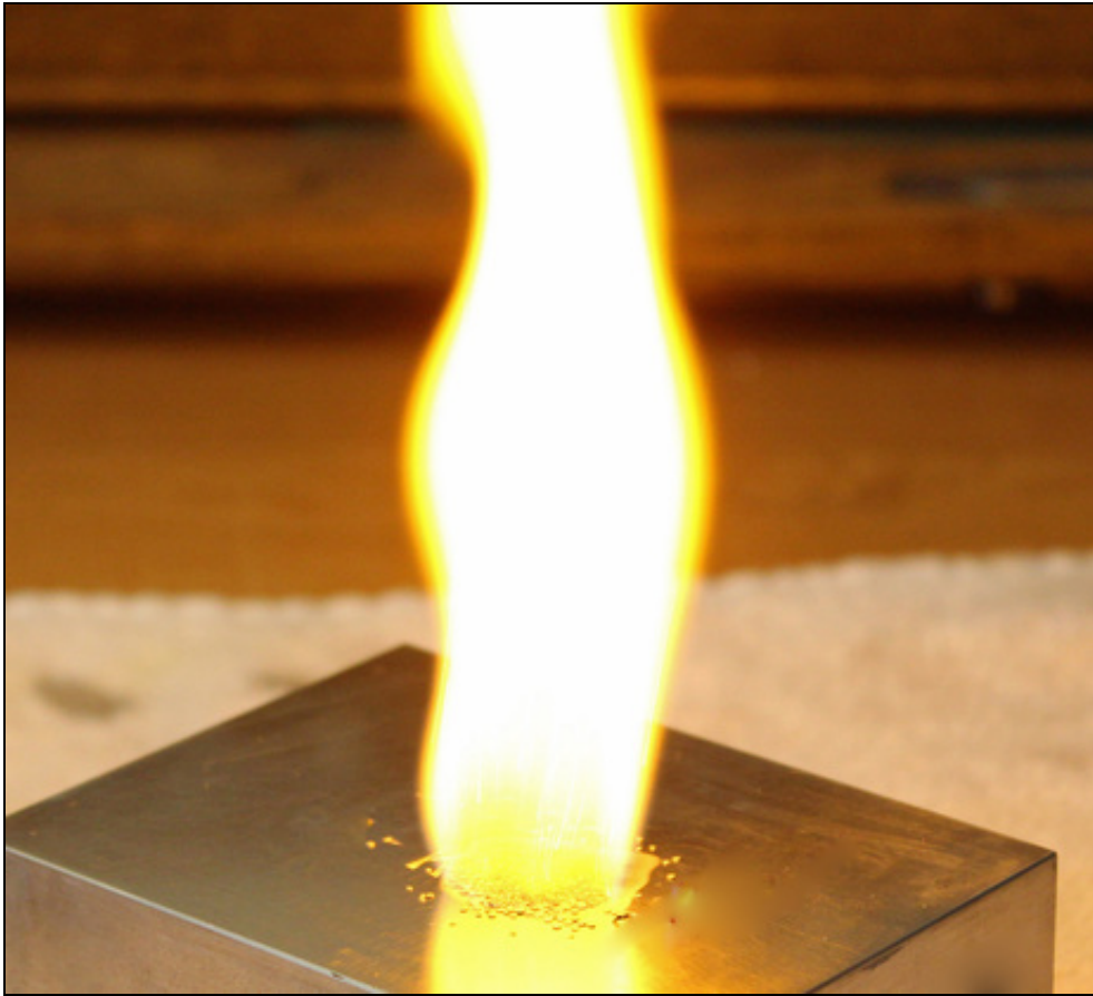
CCI powder burning from .22lr loading.
