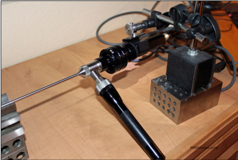
Sony camera hooked up to the borescope.
