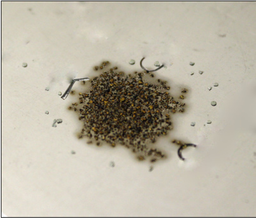
CCI powder after combustion.
