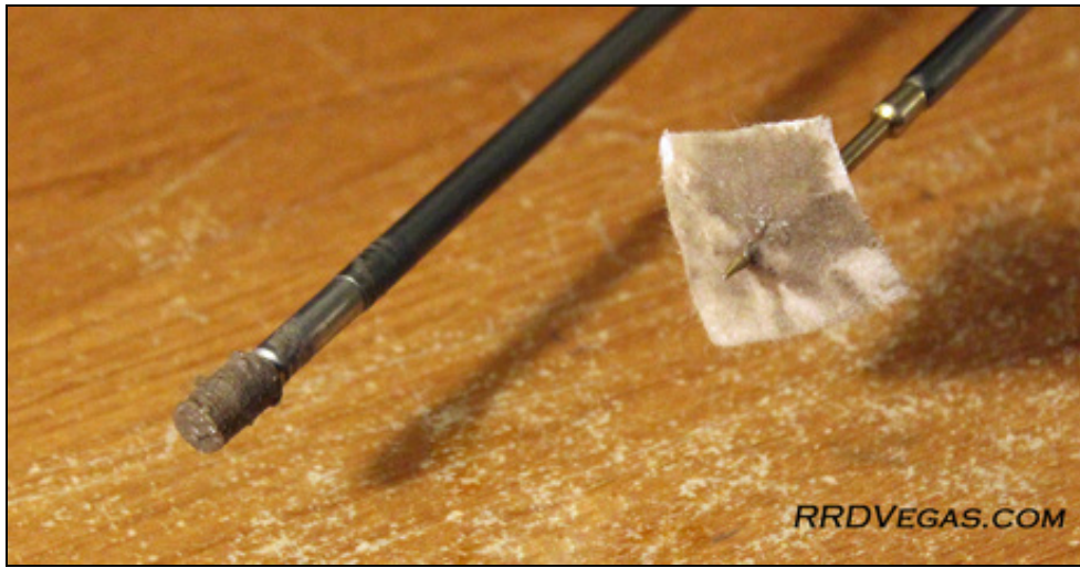
JB Bore Paste on a patch and felt pellet.
