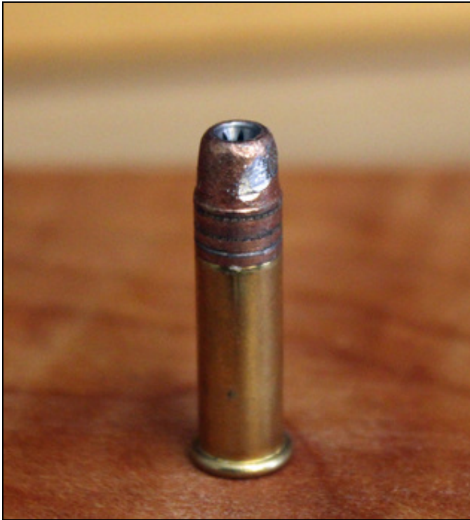
Thin copper plating found on most high-velocity 22lr.
