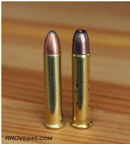
Copper Jacket (l), Copper Plated (r)
