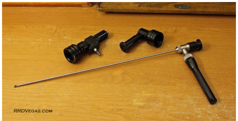
Borescope, Sony camera, and angled eye piece.
