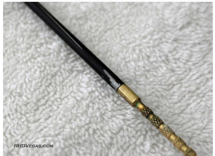
Peeling of the plastic coating and a scratch from the ejector.
