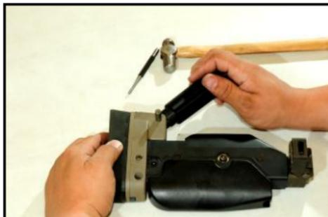
against the spring tension, moving the Monopod into the desired position, and then releasing the barrel of the monopod. The Monopod will retract to the rear when properly locked. Ensure the Monopod is firmly locked into position before firing.
