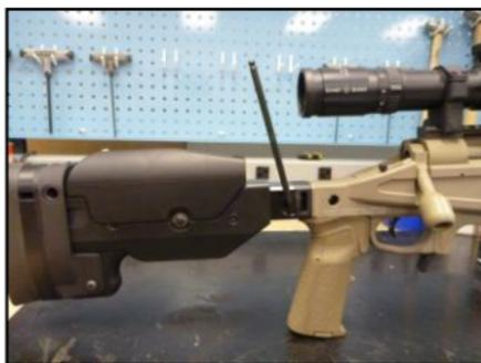
Using a SABER Field Multi-Tool or 3/16" hex wrench loosen the anti-vibration fastener approximately four turns.
