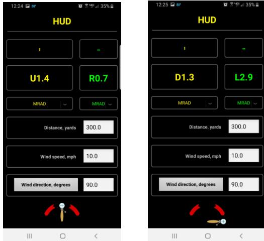
**Hide Angular Measurement(s)** - On the home page, press and hold the *turret adjustment* column number, e.g., MOA, if the shooter wants that measurement not to be visible or to reappear.
