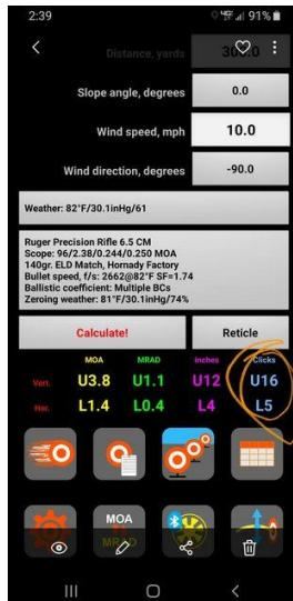
**Cartridge Quick-Change Option** - On the home page, press and hold the *Rifle and Cartridge Information* to present a drop-down menu of available cartridge loads.
