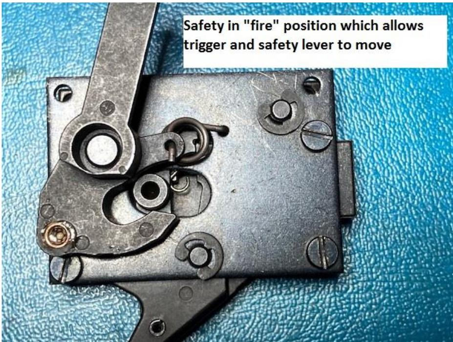
Image of trigger group with main safety and side cover removed so you can see how everything lines up. The brass object holding it is a small vise I had. It helped keep things in place while I poked and prodded.
