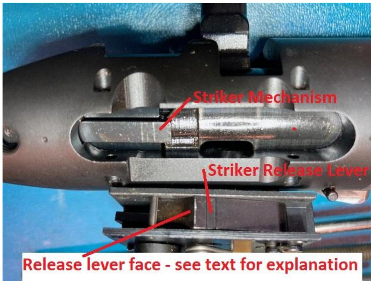
Once the bolt is cycled the front edge of the striker mechanism pushes forward against the release lever face. When the trigger is pulled, the sear will release allowing the striker release lever to drop down out of the way immediately allowing the striker to move forward and hit the primer and make the BOOM we love to hear.
